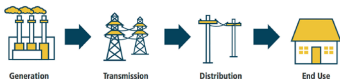
Figure 1-10. Traditional One-Way Flow Electricity Supply Chain 75 "The power grid was traditionally designed to move electricity from large generators to end users. Arrows represent power flows."
